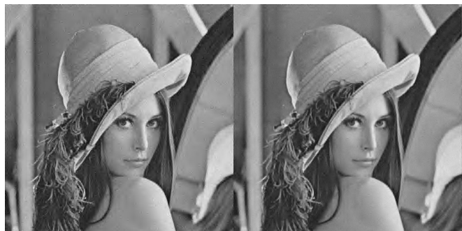
Fig. 11. Comparison of IHT reconstruction (left, PSNR 31.1 dB) and ARIHT (right, PSNR 31.9 dB) . \sigma_e = 10 , undersampling ratio m/n = 0.43
