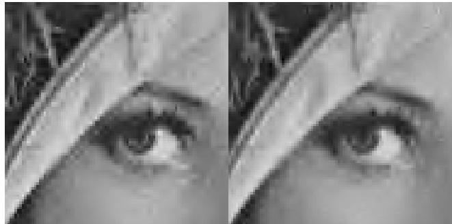
Fig. 12. Closeup of comparison from Figure 11; IHT reconstruction (left) and ARIHT (right), \sigma_e = 10 , undersampling ratio m/n = 0.43
